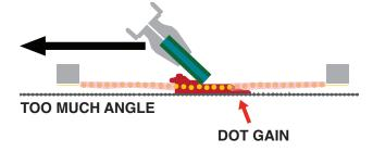
On automatic presses, start with a squeegee angle between 10–15 degrees. On manual presses, begin
