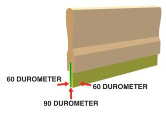
The outside durometer helps to create a softer, smoother ink deposit and is less likely to disturb surface fibers. White inks and inks with high white content, like yellows, benefit from 60/90/60 squeegees. For dark inks, 70/90/70 helps to hold finer detail.
