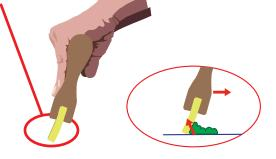
Be sure to flood the screen before committing to your print stroke. Load your screen stencil with the flood stroke and then with adequate pressure, print with the print stroke.. The goal is to deposit the ink onto the substrate while simultaneously sheering the top of the ink off.
